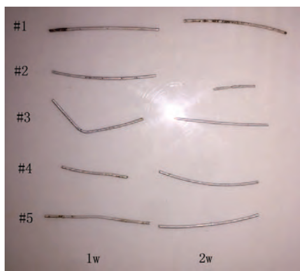
Fig. 2. Macroscopic degradation in Mg alloy pins after 1–2 weeks in vivo .
