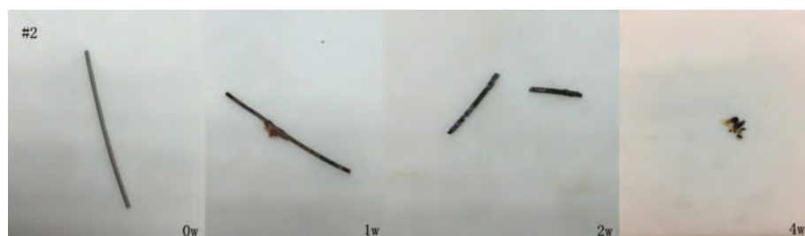
Fig. 3. Macroscopic morphology of Mg alloy pins of group 2 after 0, 1, 2, and 4 weeks in vivo .
