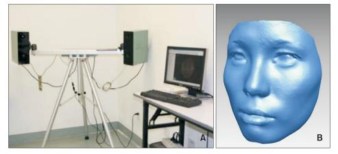
**Figure 1. A**, The three-dimensional structured light scanning system; **B**, initial three-dimensional facial image.
